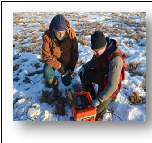
Fig. 3: photo of resistivity survey in progress
