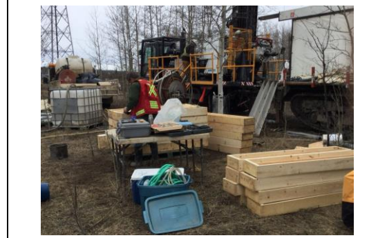
Fig. 4: Photo of drilling and analyses of drill core to confirm the finding of the resistivity survey.
